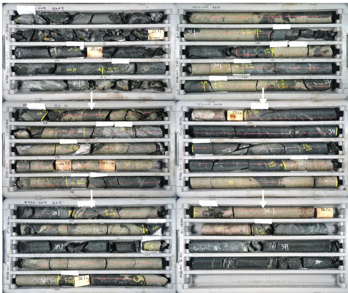
Figure 1. Core photos showing the mineralized zone from 24.6 to 36.3 m in hole KY26-009: 11.7 m of 1.92 g/t Au, 1.71% Cu, 12.5 g/t Ag, and 0.67% Zn.
