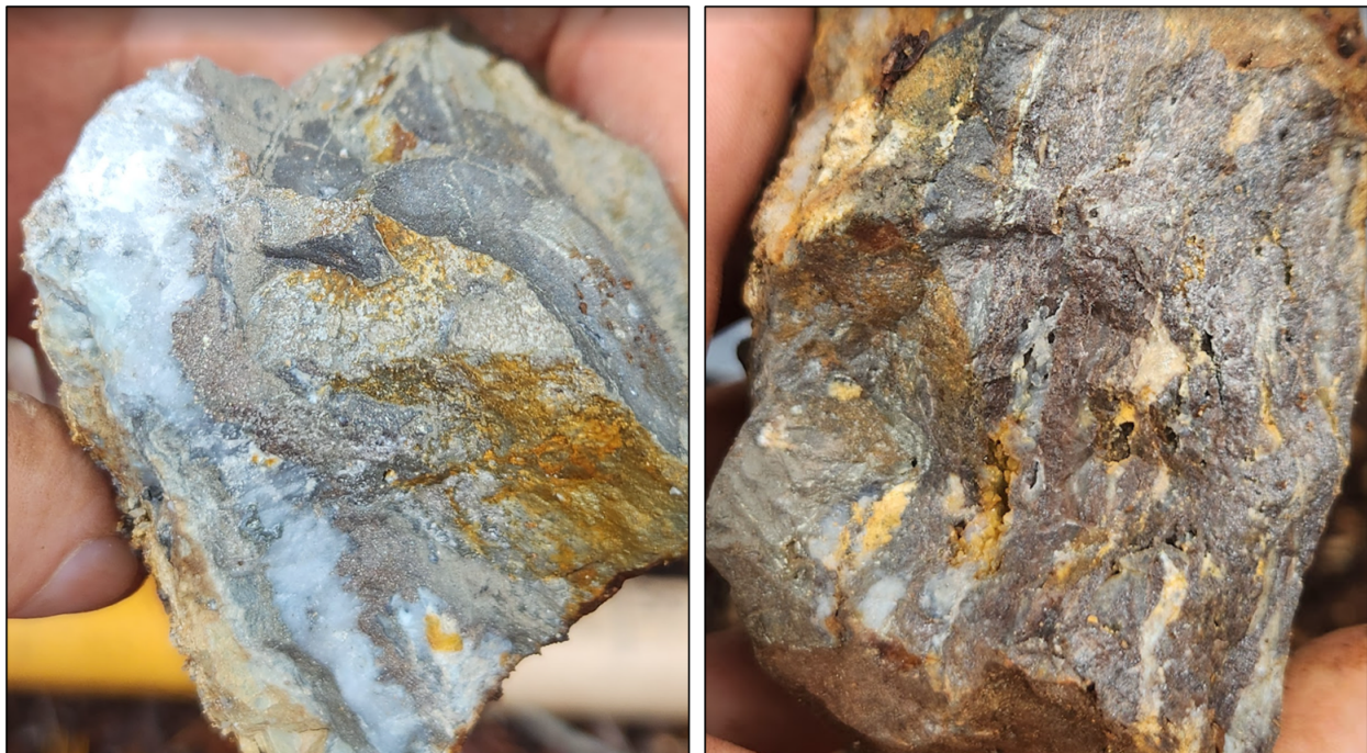
Figure 15. Photos of Lost Lake mineralization taken from the westernmost trench. Mineralization is generally parallel to bedding and occurs as fine-grained dark reddish brown sphalerite, pyrite, galena, and possible sulfosalts, and contains host rock clasts locally. Foliation-parallel quartz veins may remobilize and recrystallize sulphides.
