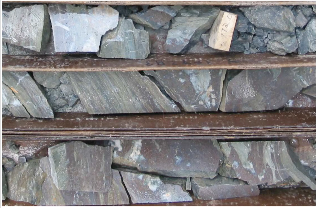
Figure 13. Core photo from MD04-001 (at 52 m) showing massive sulphide. Dark reddish sphalerite interlayered with altered tuffaceous material.
