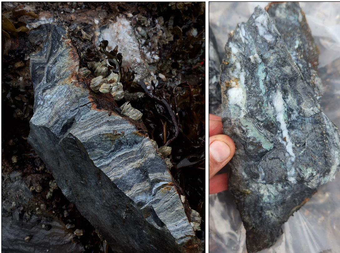
Figure 12. Photo of grab samples of Mad Dog mineralization. Left: finely banded massive sphalerite, galena, \pm sulfosalts in quartz-sericite-ankerite altered tuffs. Right: massive fine-grained sulphide with quartz bands and green mica.
