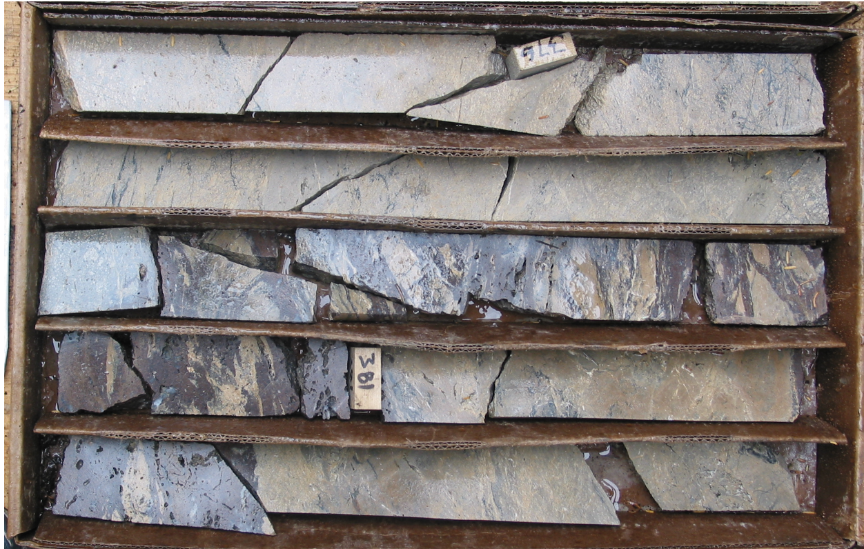
Figure 16. Core photo from LL04-002 showing dark reddish-brown sphalerite-rich mineralization within tan sericite- and carbonate-altered tuffs.
