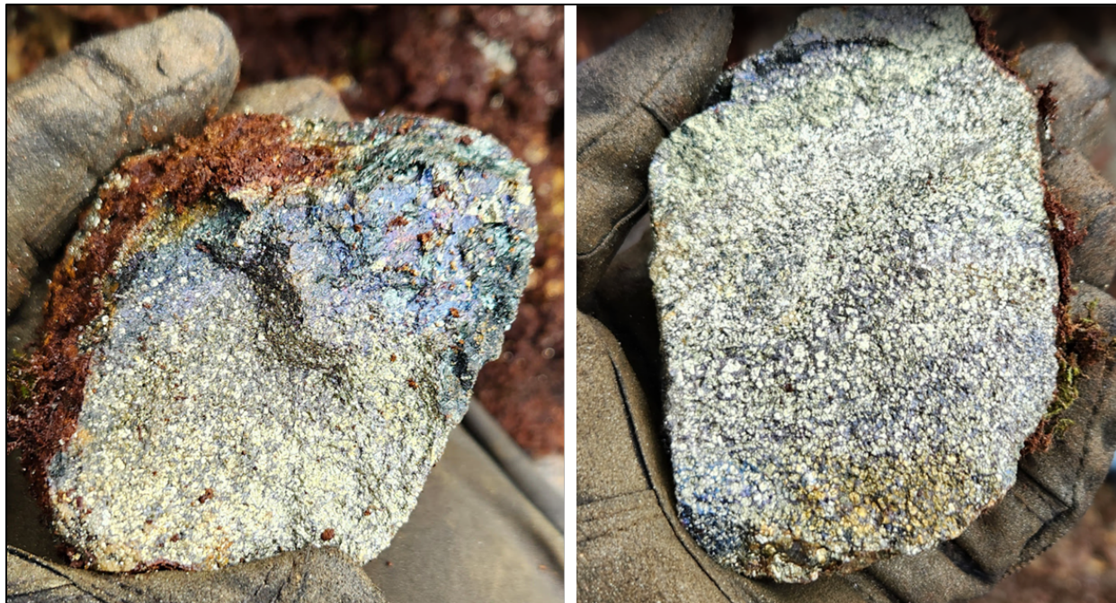
Figure 20. Example of massive sulphide from Adit 6 showing sulphide banding with pyrite, chalcopyrite, and bornite. Photo is from an area sampled as a 1.2m chip (M830559) that returned 6.2 g/t Au, 83.7 g/t Ag, 11.8% Cu, and 6.1% Zn.
