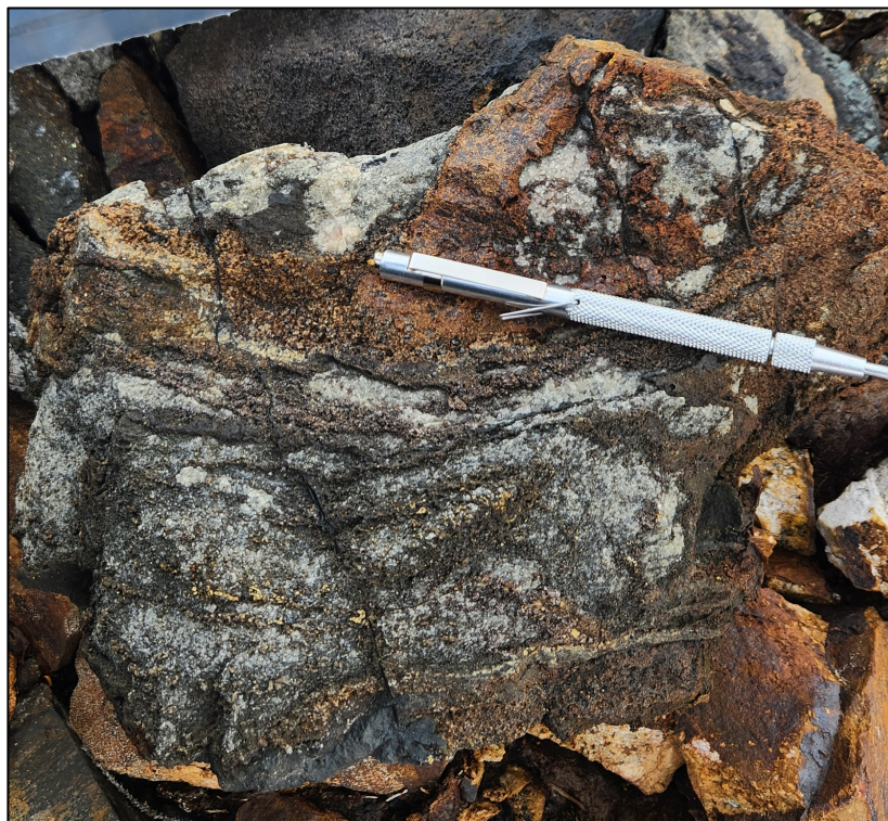
Figure 23. Massive carbonate ore with pyrite, dark reddish-brown sphalerite, and magnetite bands. From a test pit south of the Khayyam mine (Figure 15). Sample returned 1.1 g/t Au, 1.6 g/t Ag, 7.8% Zn, and 0.1% Cu.
