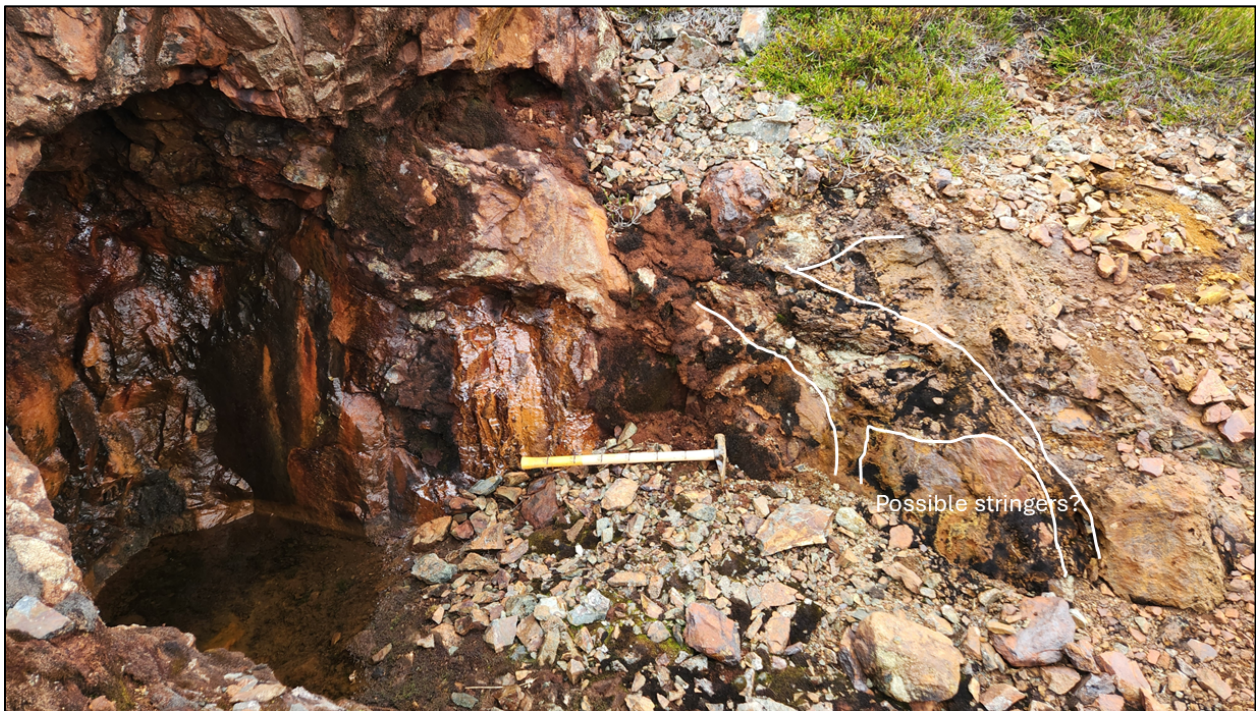
Figure 19. 'Adit' No. 6 at Khayyam. Possible sulphide stringers (right) adjacent to massive sulphide (left) within the excavated section. A 2.2 m chip sample from the adit returned 3.7 g/t Au, 54.9 g/t Ag, 8.1% Cu, and 6.5% Zn (Table 6).
